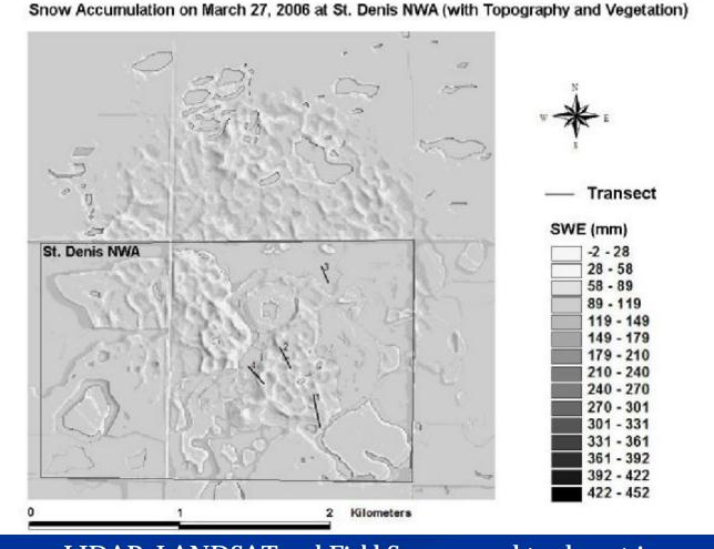
LIDAR, LANDSAT and Field Surveys used to charactrize terrain and roughness
