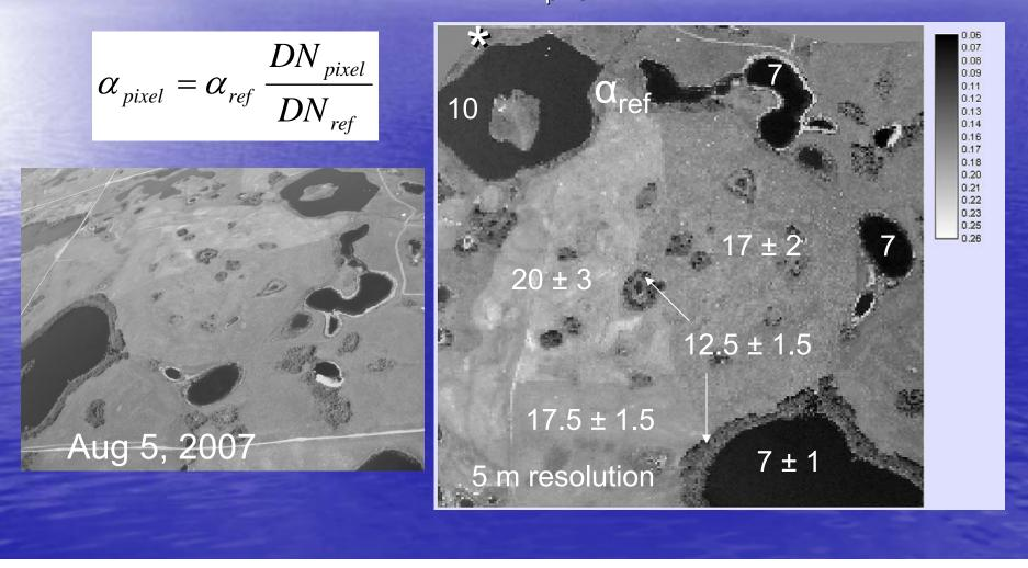
Spatial Variability of L $\uparrow$  from Thermal Image • Thermal image; FLIR Camera (7.5 - 13 µm) L $\uparrow$  =  $\epsilon\sigma(Ts+273.15)^4$ ;  $\epsilon$  = 0.98;  $\sigma$  = 5.67 x 10<sup>-8</sup>
