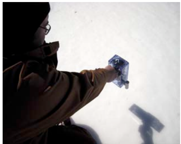
Photograph of the acoustic snow water equivalent gauge being deployed to send and receive a sound wave through the snowpack. The device has on board signal processing to estimate depth and density from the transformation of a frequency-swept sound wave returning from the snowpack.
