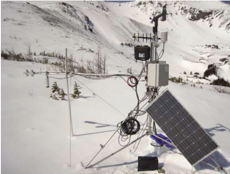
A photograph of the meteorological station and time lapse camera at Marmot Creek Research Basin in the Canadian Rockies. The station is used to provide hydrometeorological data to run and validate blowing snow, snowmelt and snow covered area depletion models.
