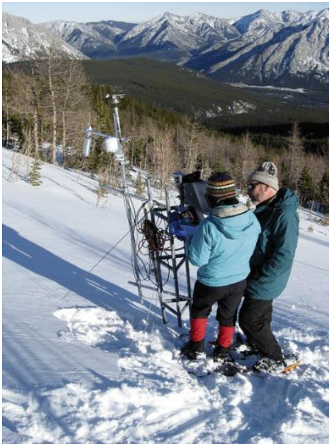
Field technician May Guan, left and Dr. John Pomeroy download information from a datalogger at the south side outlier station on Fisera Ridge.
