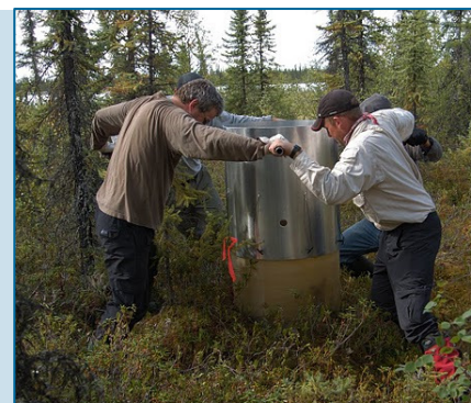
Sampling of the undisturbed peat cores in the Scotty Creek basin
