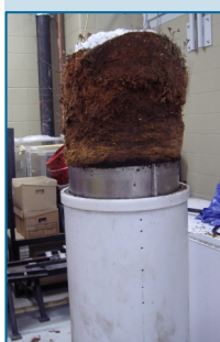
Undisturbed core being inserted in experimental drums
