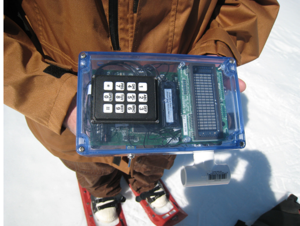
Figure 2: Second prototype snow sonar device deployed at the Rocky Mountain sites.
