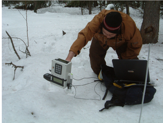
Figure 1: First prototype snow sonar device being deployed at the Yukon sites.
