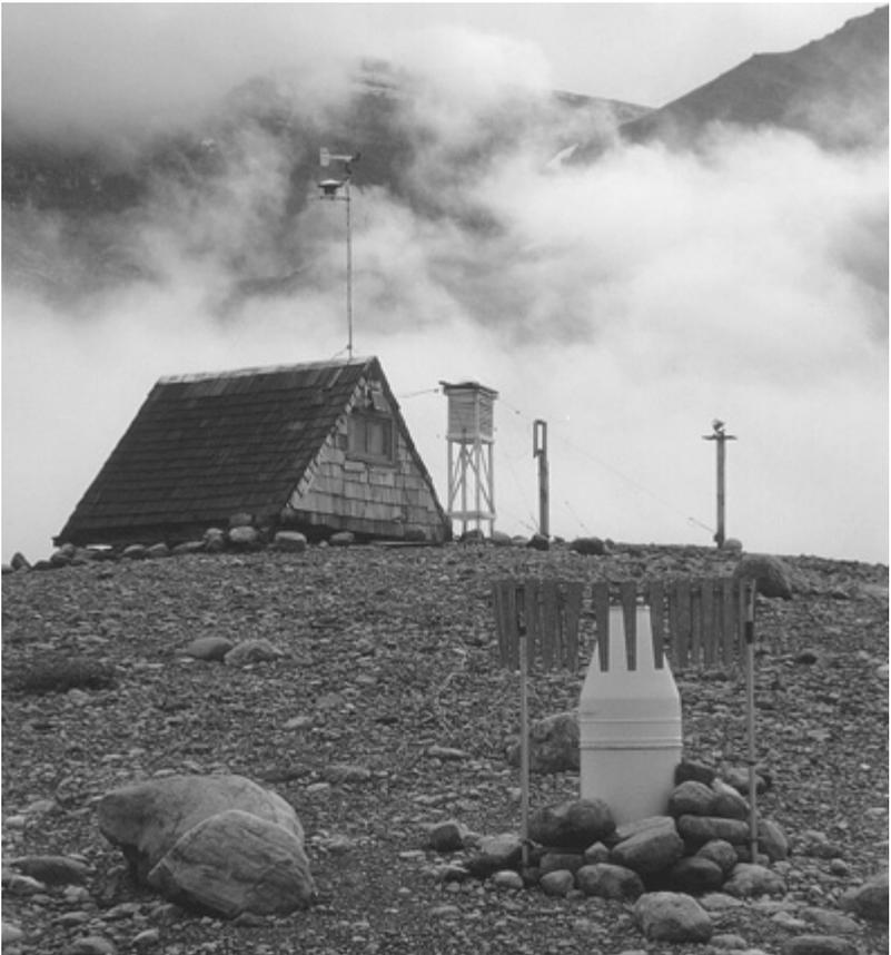
**Figure 1.** Peyto Glacier weather station, showing sensor locations for air temperature, solar radiation and shielded precipitation gauge.
