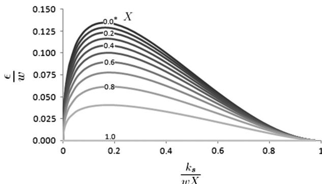
Figure 2. Dimensionless error in the linear approximation,  $\varepsilon$ , as a function of dimensionless conductivity, normalized to the dimensionless time parameter,  $X$ . The curve labelled 0.0\* is the limit of  $\varepsilon$  as  $X$  approaches zero
