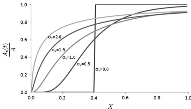
Figure 4. Evolution of basin surface saturation for various degrees of heterogeneity in hydraulic conductivity.  $X$  is the dimensionless time parameter
