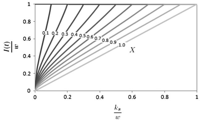
Figure 1. Dimensionless Green-Ampt infiltration rate as a function of dimensionless conductivity. Individual curves correspond to snapshots of dimensionless time,  $X$ , which progresses from  $X = 0$  at  $t = 0$  to  $X = 1$  at  $t = \infty$ . For the definition of  $X$ , see text
