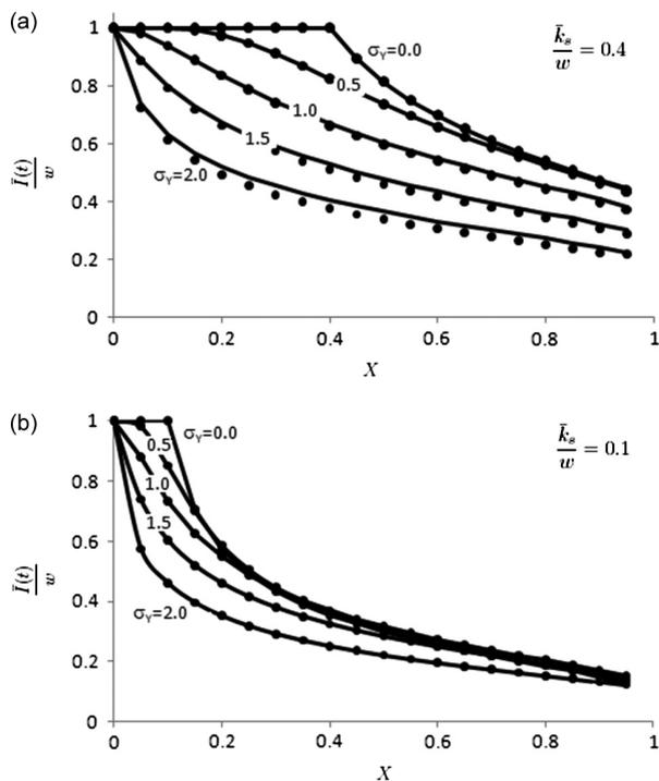
Figure 5. Semi-analytical (solid) and Monte Carlo (circles) dimensionless infiltration for heterogeneous domains with an average conductivity,  $\bar{k}_s$ , of 1.6 cm/h (a) and 0.4 cm/h (b), and rainfall rate of 4 cm/h. Variability in conductivity is quantified using the normalized standard deviation of log-conductivity,  $\sigma_Y$ , which is here varied from 0 (homogeneous) to 2 (highly heterogeneous)
