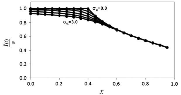
Figure 6. Analytical (solid) and Monte Carlo (circles) dimensionless infiltration curves for a homogeneous domain with spatially variable initial conditions. Here,  $k_s = 1.4$  cm/h and  $w = 4$  cm/h
