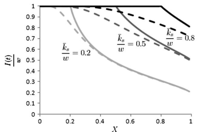
Figure 3. Evolution of dimensionless infiltration rate with the dimensionless time parameter for standard (solid) and upscaled (dashed) GA solutions. Three different ratios (0.2,0.5,0.8) of average conductivity to rainfall rate are depicted. The coefficient of variation ( $k_s/\sigma_k$ ) for all three upscaled models was kept fixed at 0.5
