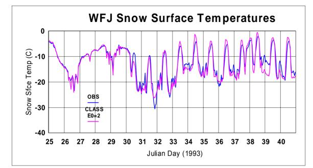
Significant improvement in snow surface temperatures with  $E_0 = 2 \text{ W m}^{-2} \text{ K}^{-1}$  and albedo modified to represent observed values (CLASS albedo too low by ~0.15 at this site)
