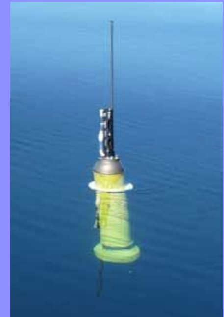
An APEX buoy which rises to the surface every three days to transmit temperature, depth and conductivity via satellite.
