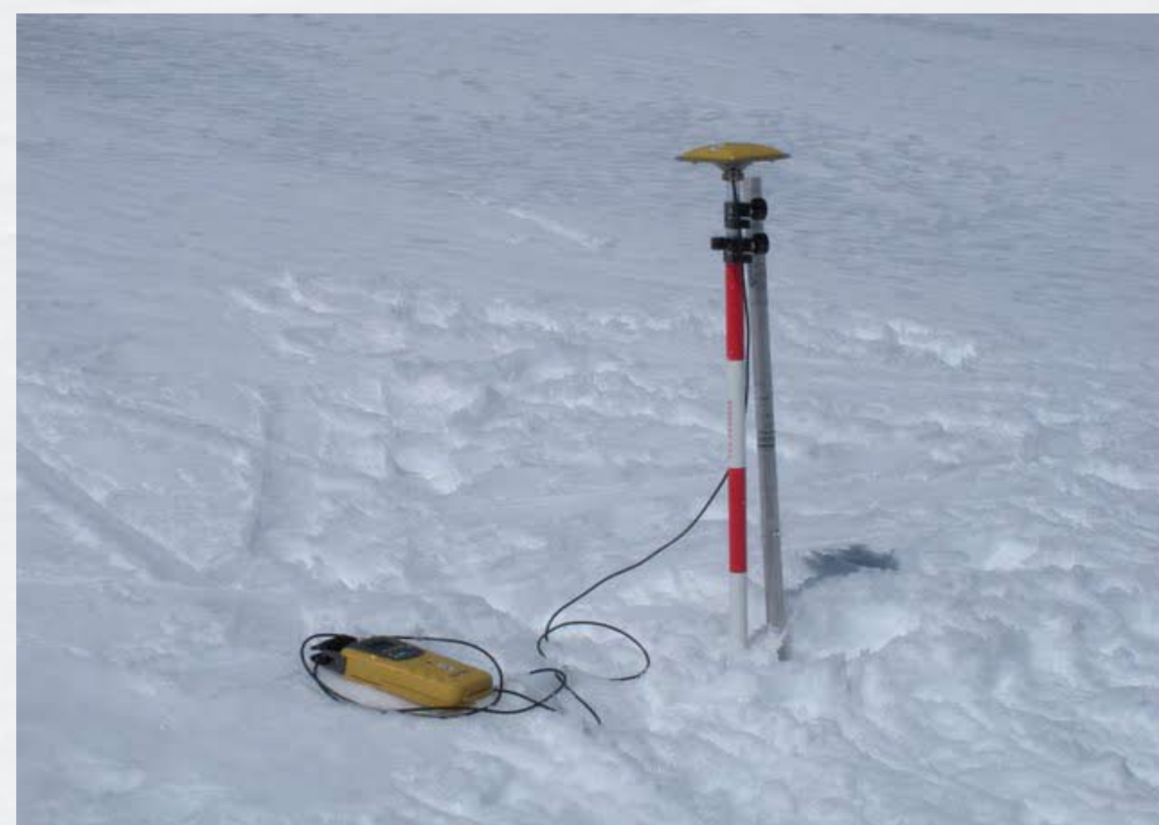
Figure 5: A rover antenna recording the position of one of the velocity stakes.
