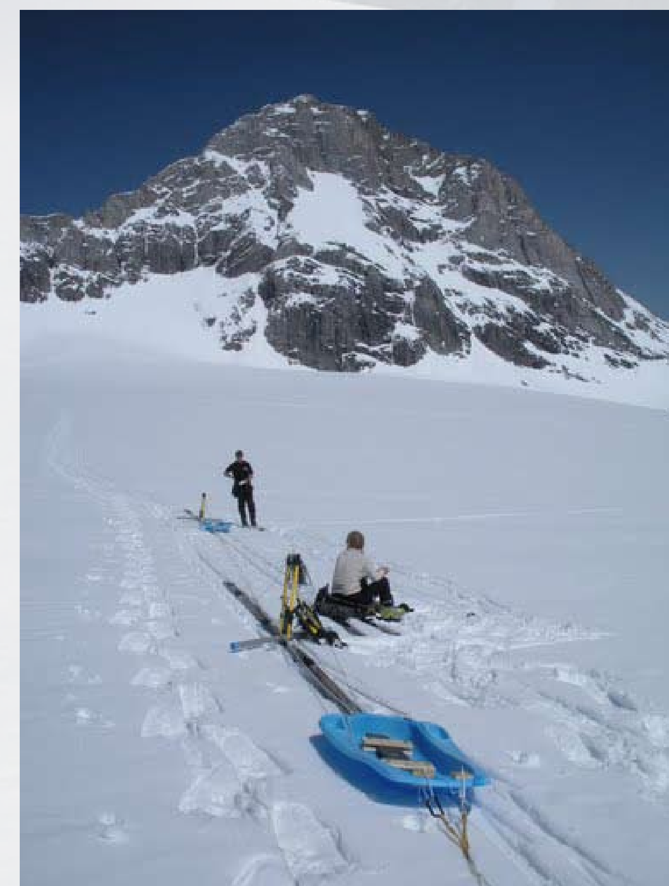
Figure 6: Orientation of GPR antennas during data collection. The direction of drag is towards the bottom of the photograph.
